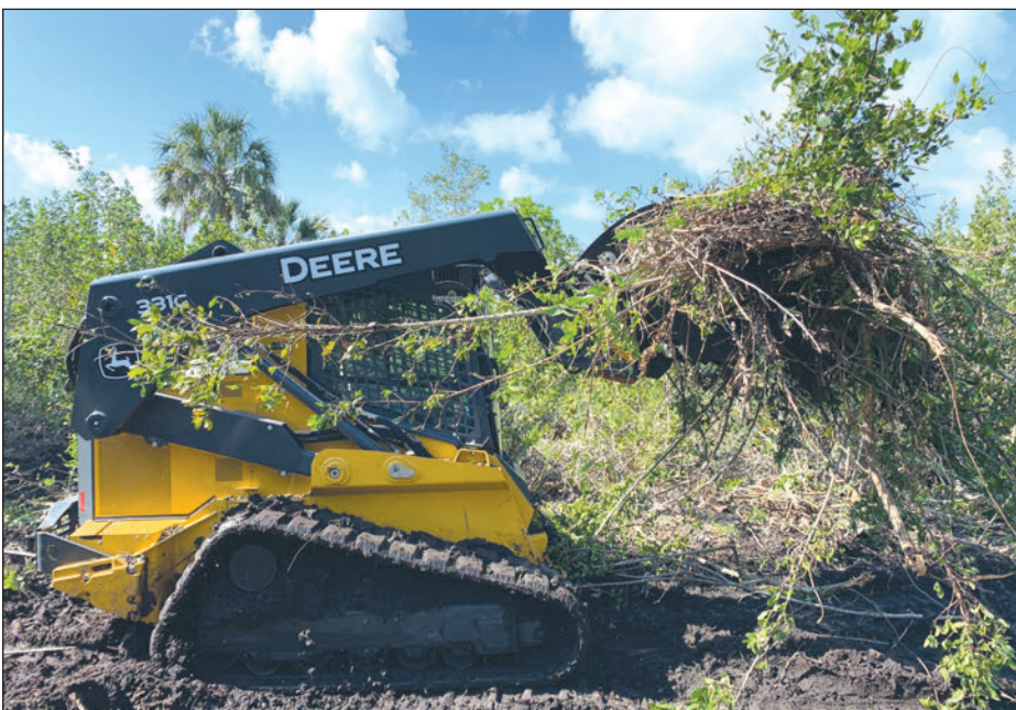
The root rake grapple attachment allows the team to grab exotic vegetation, debris and downed trees and move them to piles. Here it is carrying a Brazilian pepper tree to a pile of debris after ripping it out of the ground, roots and all.
